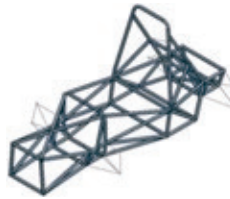
Fig. 2. Spatial construction of the analysed frame.
